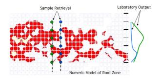
The relevance (and this is an example from the numerical model) is an explanation for the considerable variation when testing soils, even when bores are sunk close to one another - see above. Two bores sunk within 1mtr can deliver very different results.
