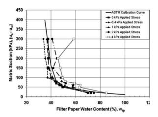
The findings confirm the importance of using the correct calibration curve - the one that matches what actually happens in the laboratory. The authors suggested using a 1kPa loading to ensure the correct contact is made between the sample and the paper.
