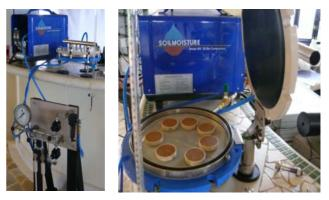
They have undertaken their own calibration using six batches of 12 No. 50mm diameter x 10mm high clay samples placed in the pressure membrane extractor and taken to suctions of 100, 250, 500, 750, 1,000 and 1,500 kPa.
