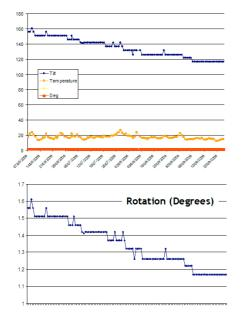
By plotting temperature alongside movement, we can discount it as a cause. Second, because we are measuring fine movement we can detect it much quicker than say, crack or level monitoring.
