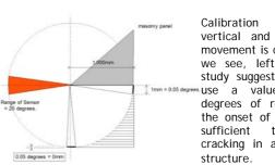
between vertical and rotational movement is complex as we see, left, but our study suggests that we use a value of 0.2 degrees of rotation as the onset of movement to cause cracking in a domestic
